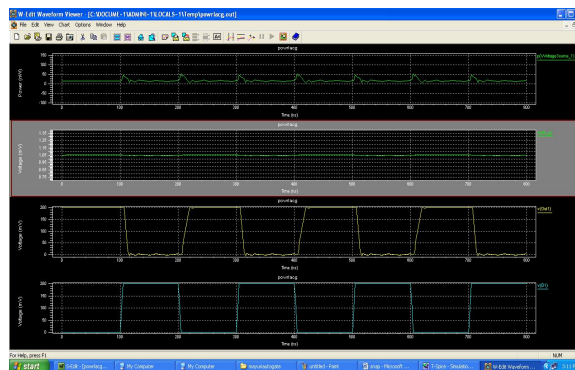
Fig. 6 Look ahead clock gating waveforms.
